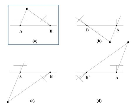
Only 1 of the 4 solutions is physically correct, i.e. the 3D point appears in front of both cameras.
